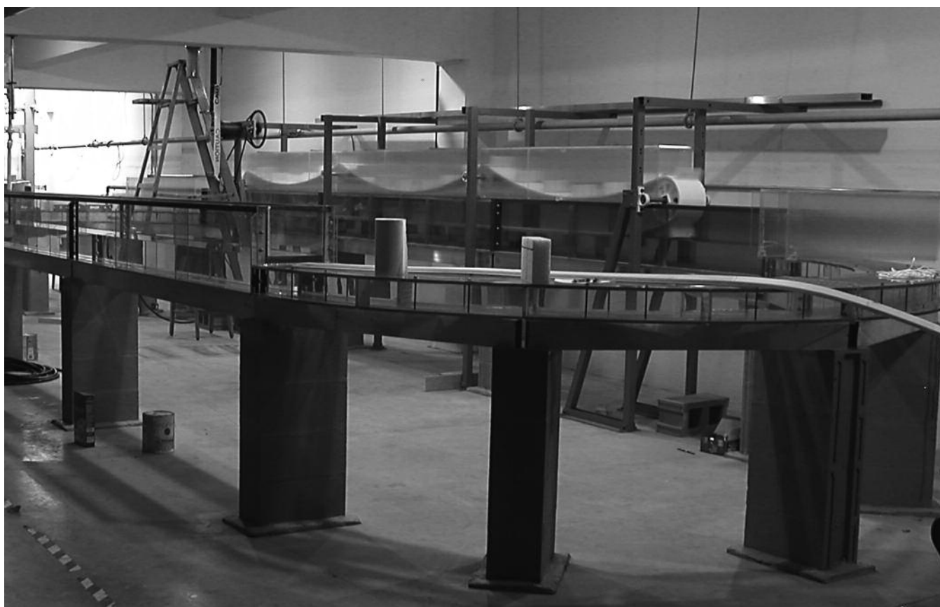
Figure 1. The current flume lab at Indiana University with two racetrack flumes. Each flume is 10.5m x 3.5 m in size and has a paddle-belt drive. They have been specially designed for experiments with muddy suspensions and avoid the destruction of flocculated materials, a drawback of other recirculating flume designs.
