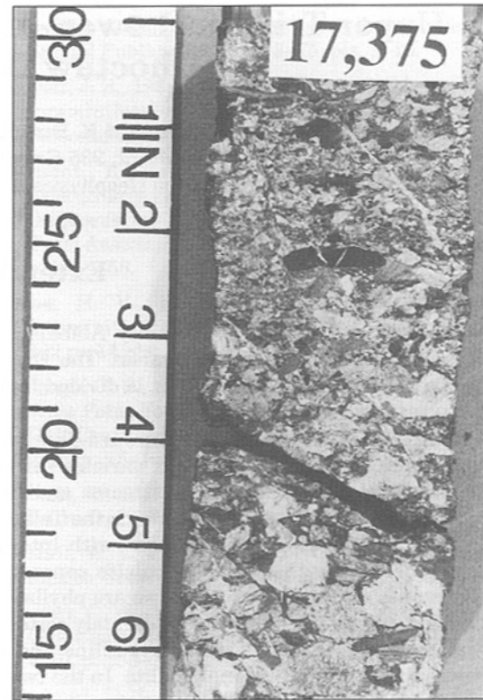
Figure 2. Upward-fining conglomerate channel deposit. Light-colored clasts are quartzite; dark elongate clasts are hematite-stained phyllite and schist.
