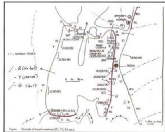
Fig. 2. Rockfall hazard map, Tambun, Ipoh.
