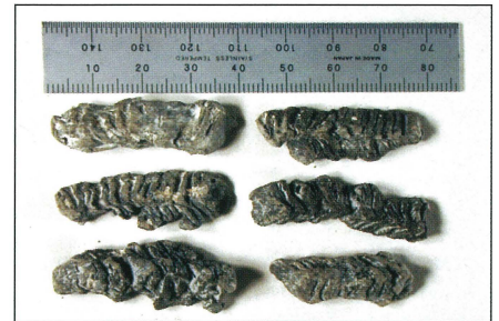
Reactive shale cuttings drilled with BarOmega. Image provided by Halliburton Baroid.
