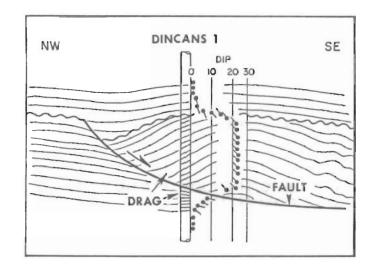
Diagrammatic illustration of rotated slump block in the downdip Yegua turbidite channel sandstones, Cities Service Dincans 1, Gas Unit 1, Toro Grande field, based on core examination and dip-log interpretation. Slumped section is about 60 ft (18.3 m) in thickness.
