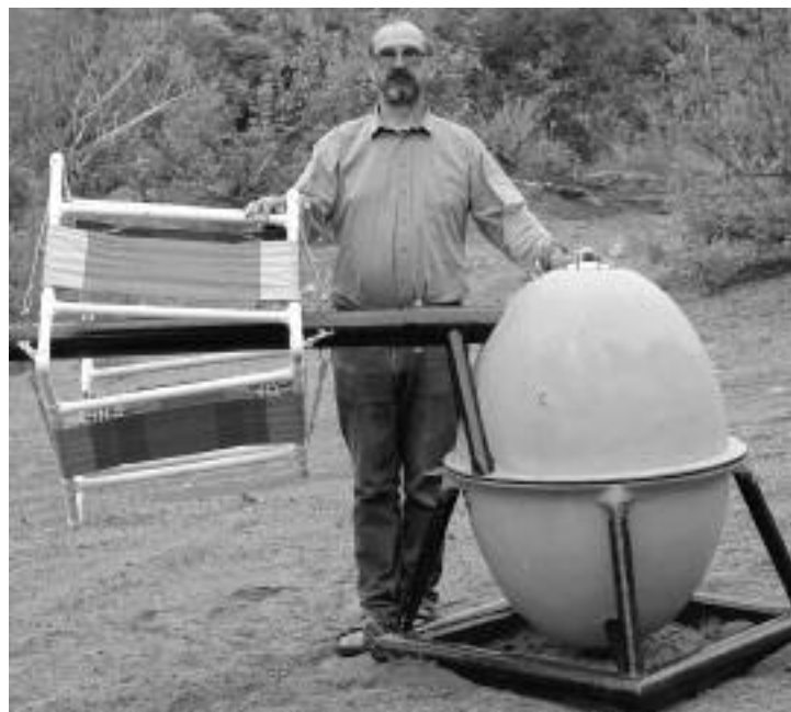
Figure 2 - Geotech's airborne AFMAG system in field trials in Sudbury, Ontario with the principal designer, Dr. Petr Kuzmin.
