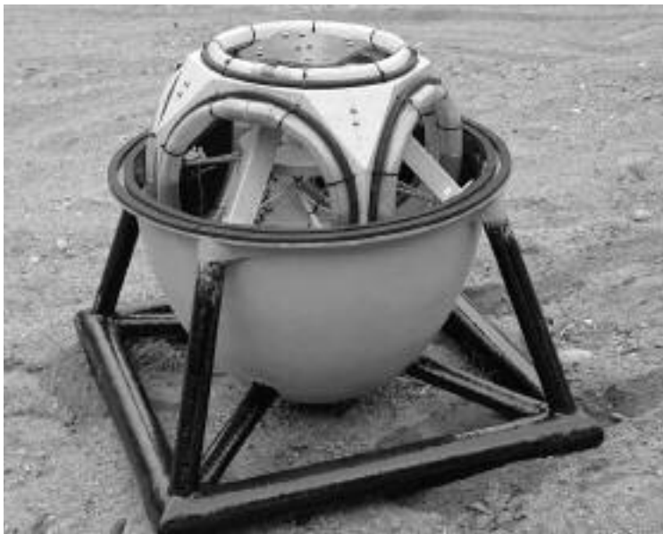
Figure 1. AFMAG unit interior showing the three orthogonal coils, damping mechanism and suspension.
