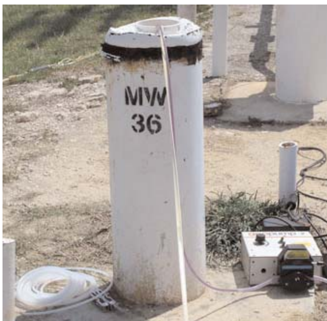
Groundwater monitoring conducted during pilot oxidant injection test. The purple color in the purging lines indicates the presence of the oxidant in groundwater.
