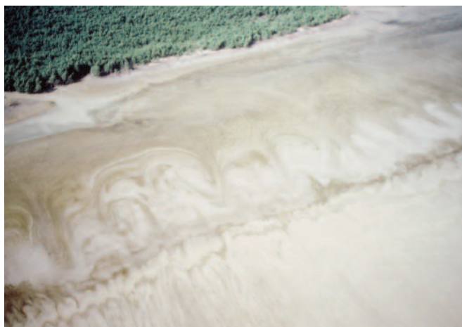
Aerial view of exposed mud bank at low tide showing surface flow features within the fluid mud. Approximate width of view is 500m.
