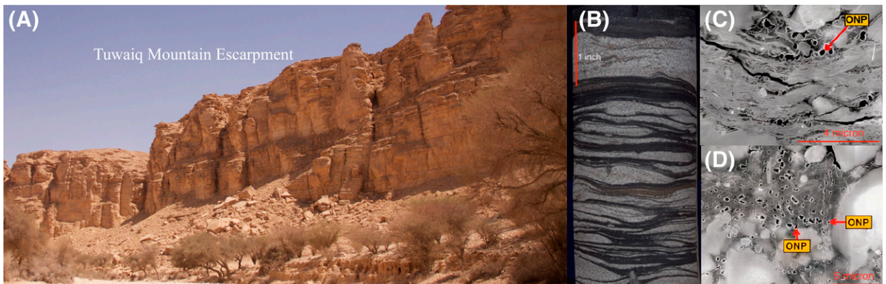
Figure 4. (A) A Tuwaiq Mountain Formation escarpment along the Riyadh-Makkah highway. (B) A shale core having an interbedded organic-rich layer and carbonate layers. It represents the effect of changing sea level in the carbonate depositional platform. Source: Ferri et al. (2011). (C, D) Scanning electron microscopy images of Tuwaiq Mountain source rock showing the distribution of organic matter. The dark specks are made of kerogen. These specks are disconnected at the microscale. Source: Hakami (2016). ONP = organic nanopores.
