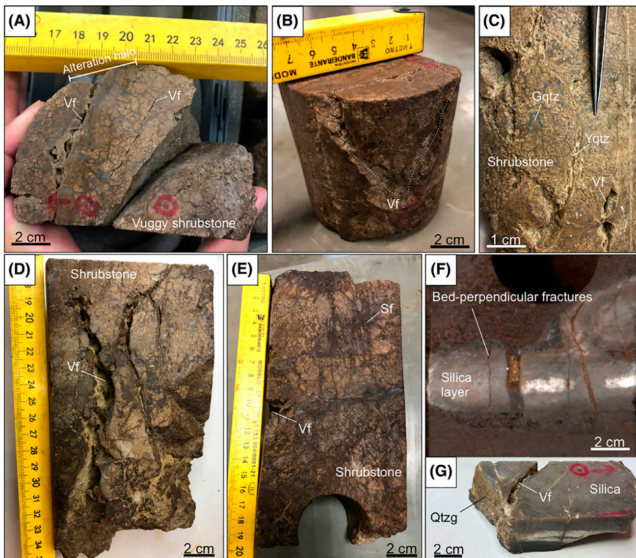
Figure 3. Fracture and dissolution features observed in the core from well A. (A) Vuggy fracture (Vf) cutting the shrubstone host rock with alteration halo. Most primary pores of the host rock are filled with grayish quartz. Host rock is commonly observed with vuggy aspect. (B) The Vf crossing the core. Vugs are coated with up to 1-mm-sized euhebral quartz crystals. (C) The vuggy fractures filled with yellowish quartz (Yqtz) and shrubstone host rock cemented with grayish quartz (Gqtz). Sparse vugs or geodes filled by quartz crystals are observed in the host rock. (D) The vuggy fractures with centimeter-sized aperture coated by euhebral quartz. (E) Narrow small displacement fault (Sf) swarm, with cataclastic fill. (F) Silica layer bearing bed-perpendicular opening-mode fractures. (G) Silicified spherulitstone host rock and open Vf with euhebral quartz. This fracture is associated with centimeter-sized quartz geodes (Qtzg).
