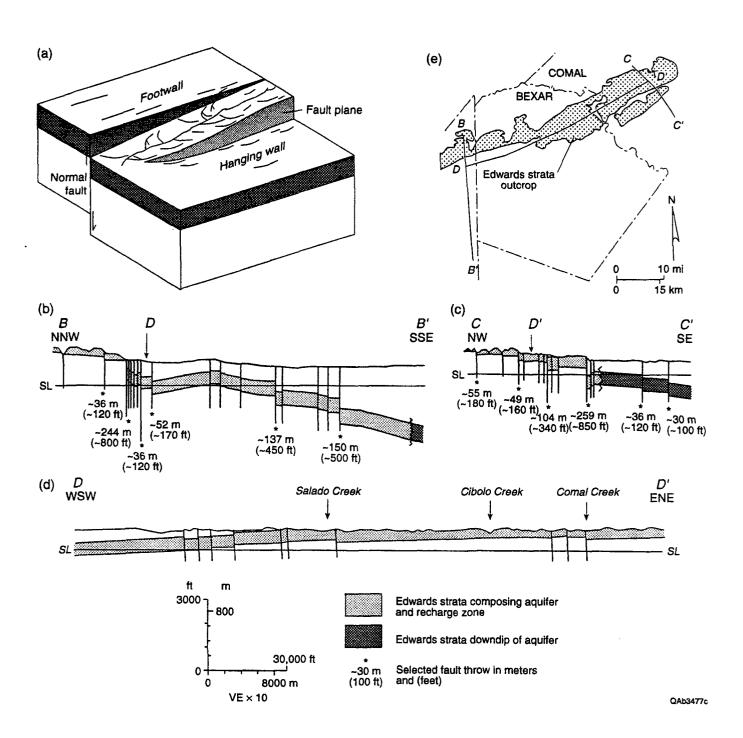
Figure 1. (a) Schematic block diagram of relay ramp. Folded aquifer strata in ramp are highly fractured locally and serve as a highly transmissive pathway where offset on major faults has otherwise reduced aquifer continuity. (b) and (c) Structural cross sections of Edwards strata cut by master faults of the San Antonio relay ramp. (d) Structural cross section along axis of relay ramp. (e) Location of cross sections.
