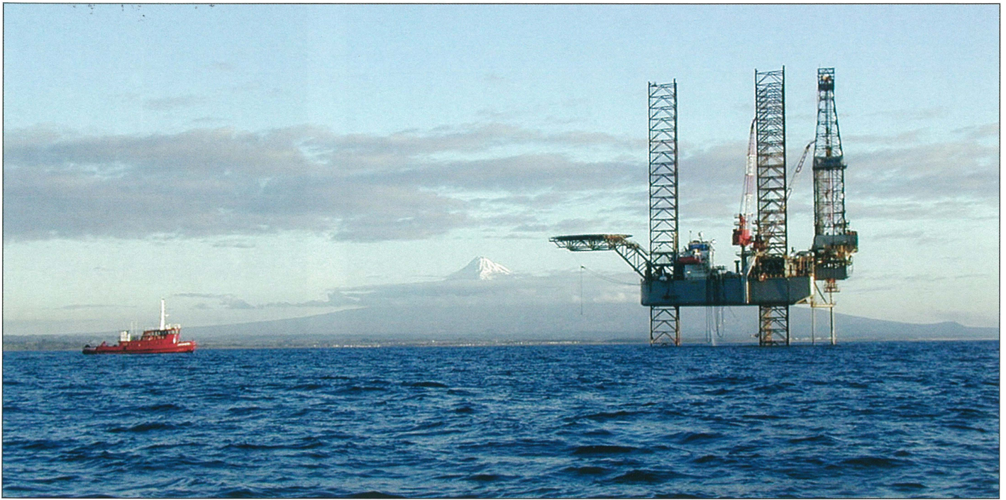
The ENSCO-50 jack-up rig drilling Pohokura-1, with a backdrop of Mt Egmont/Taranaki.
