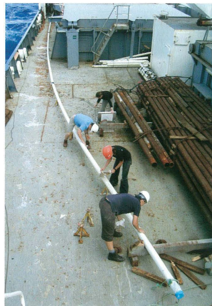
Labelling one of the giant (Calypso) piston cores prior to it being cut into 1.5 m long sections for splitting and sampling.
