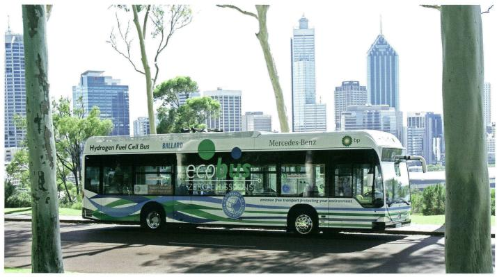
One of the three hydrogen buses being trialled in Perth, at a total cost of about \$10 million, at Kings Park. The buses have covered more than 160,000 km and carried more than 200,000 passengers since the trial began in 2004. Picture courtesy: WA Department of Planning and Infrastructure.
