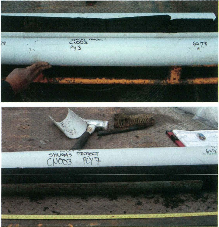
Lignite core samples from the second hole in the Clinton Phase of the drilling program.
